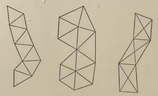
quadrilaterals only, the adjustment of each is made by Art. 80, and the sides then found from the plane angles. If it be made up of triangles, polygons, and quadrilaterals, as is generally the case, the same process may be followed, by starting at the base and treating each part in succession. Lastly the latitudes, longitudes, and azimuths are computed by the method of Art. 66 if the triangulation be a geodetic one, or by that of Art. 19 if it be plane.
